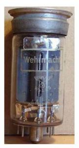
Wehrmacht transmitting tetrode capable of operation from audio frequencies up to about 120MHz. 40W anode power dissipation.
