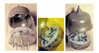
German VHF/UHF double diode, capable of operation as detector in the gigahertz region.
