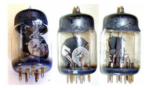
High frequency military transmitting triode, capable of CW or pulsed operation down to 35 cm wavelenght. 25W anode power dissipation.
