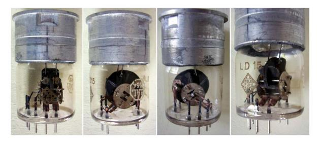
German Wehrmacht Luftwaffe transmitting triode, capable of pulsed operation as oscillator or as frequency doubler down to 45 cm wavelenght.
