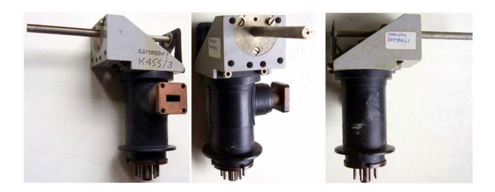
Millimeter reflex klystron. Even if it is hand marked as Raytheon K455-3, it looks very similar to the EMI series including R9518, R9521 and R9546. By the way, there is no documented tube with this code in the Raytheon production.
