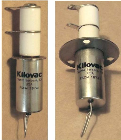
SPST 10 kV, 25A max tiny vacuum relay. 10A rated operation at DC or 60Hz, 7A at 2.5MHz, 6A at 16MHz and 4A up to 32 MHz. 2 million cycles mechanical life.
