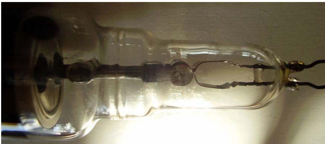
-Fig. 2 - Detailed view of the glass bulb at the transition between the large bottom chamber and the top dome containing the magnetron electrodes. The glass seal is clearly visible. Also visible the figure '44' punched on the metal baffle at left and a glass spacer across the output line at right.
