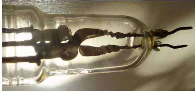
Fig. 5 - Close-up view of the internal resonating line strip, connected to the outside by means of wavy sections rigidly interlocked by a glass spacer
