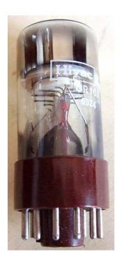
10 way register/indicator. Duodecal base. Accepted as CV5291.
