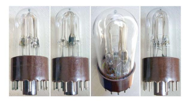
Xenon-filled arc discharge tube incorporating two EN55 stroboscopic lights that can be operated with interlaced trigger pulses. Flash rates up to 800 or even 1000 per second can be achieved. Diheptal base.
