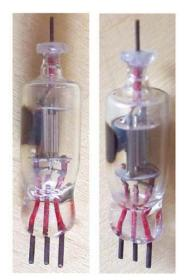
Tiny VHF/UHF signal diode.
