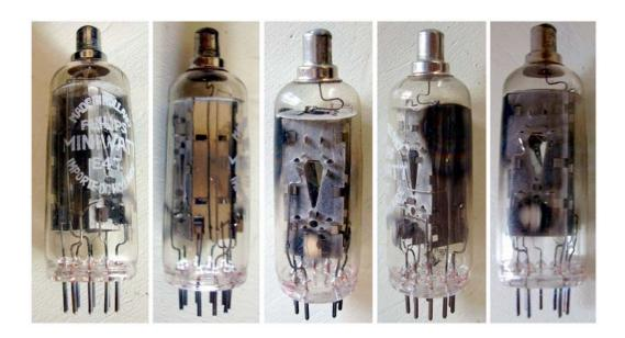
Modulated beam-deflection tube, intended for pulse generation in military or in instrumentation applications. T6-1/2 glass bulb with top skirted cap.
