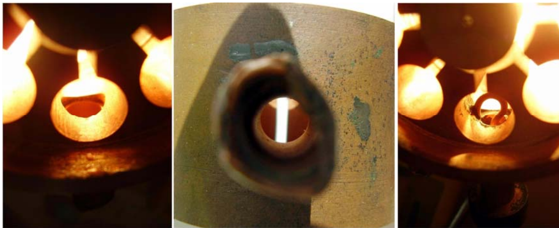
- Detailed view of the internal hole corresponding to the side copper tube. It is round and exactly in the middle of the resonator. By the way, looking from outside through the copper tube, the visible cathode surface appears in a good shape. Unfortunately in the second image the oxide surface is out of focus and just its uniform whitish look can be appreciated. On the right, the hole hosting the output coupling loop looks to have the same diameter.
