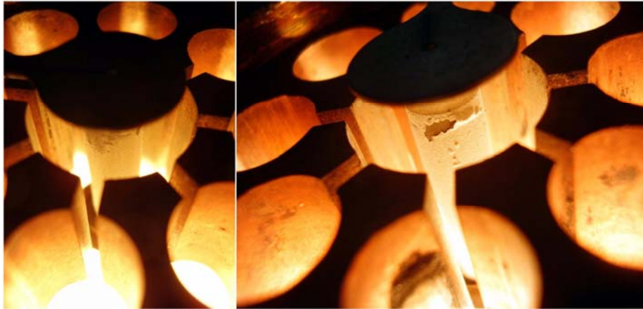
Two views of the cathode surface. The oxide layer is uniform and in good shape for about four-fifths of the cathode cylinder. Near one of the ends the layer is quite thin somewhere, leaving exposed the underlying metal. Oxide also looks swollen and detached in the small area evidenced in the image at right. One side of the cylinder ends in a flange, spot welded to the one end baffle. Not sure, but metal looks to be nickel. Click to enlarge.
