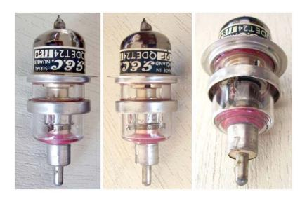
UHF planar triode capable of operation up to 2 GHz. <u>DET24</u> is the Marconi GEC code equivalent to Mullard TD04-20, both accepted under the <u>CV397</u> spec.
