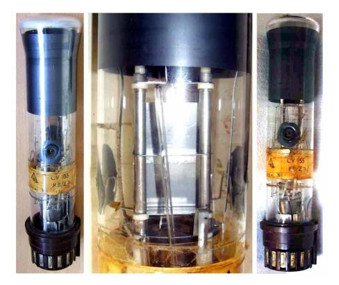
75mm green phosphor CRT. Electrostatic focus and deflection. 3 kV accelerating potential. Y deflection by side caps.
