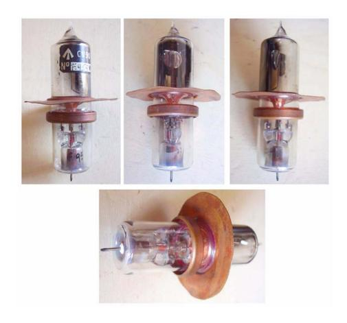
This tube, developed by STC, can be considered the forerunner of the 'rocket' style UHF triodes.
