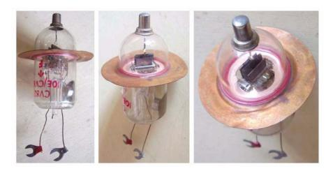
One of the very early disk seal tubes, developed by British STC as S27A and later approved as CV82. Derived from CV53, with an internal feedback between the anode and the grid circuits. Intended for use as local oscillator in receivers operating at 600 MHz, it could be used from 400 to 750MHz full ratings, giving 2W RF output.
