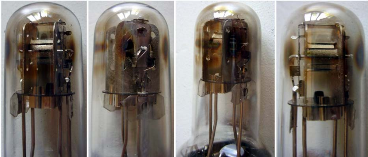
- Detailed views of the electrode structure. Click to enlarge.
