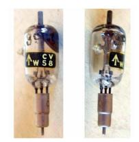
UHF diode, designed to be used in balanced or coaxial lines up to about 1GHz as a mixer or up to 3 GHz as detector.
