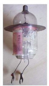
Disk seal triode with nickel anode. This kind of structure, with the grid brought outside through a copper disk, was devised for grounded grid amplifier operation.
