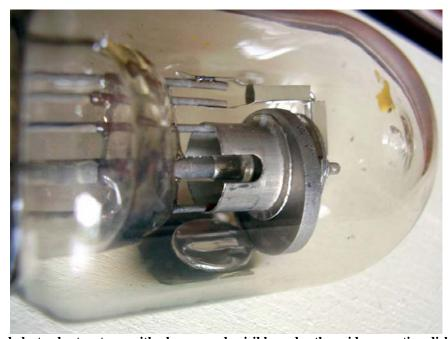
$\hbox{-} \ Reversed \ electrode \ structure, \ with \ planar \ anode \ visible \ under \ the \ grid \ supporting \ dish.}$
