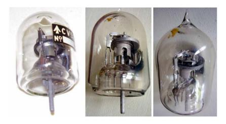
UHF triode from British GEC. 10W anode power dissipation; up to 600MHz operating frequency. Special 5-pin recessed base.
