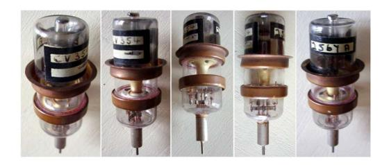
Disc seal triode designed as grounded grid amplifier inside a coaxial resonator.
