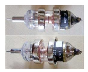
British GEC disc-seal triode for use at wavelenghts shorter than 10cm, or frequencies up to 3.7 GHz. This type replaced the <u>CV90</u> in 1945, using a similar but smaller structure to increase the frequency coverage.
