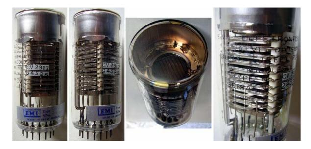
CV2317 is a 2-inch diameter top-window photomultiplier sensitive to radiation of about 4000 Angstrom wavelength. 11-stage venetian-blind type dynodes.
