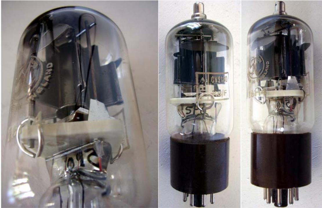
Introduced by Ediswan as VX6095, commercial code 19H4, the CV2180 is intended as high voltage rectifier or clipper. Unipotential oxide-coated cathode.
