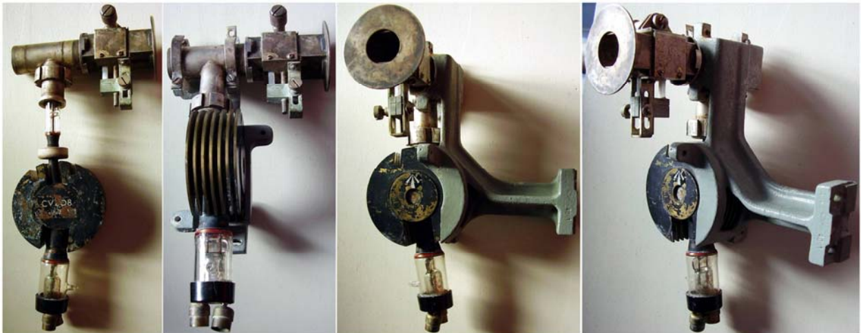
Views of the CV208 magnetron, of the waveguide transition and of the complete assembly.
