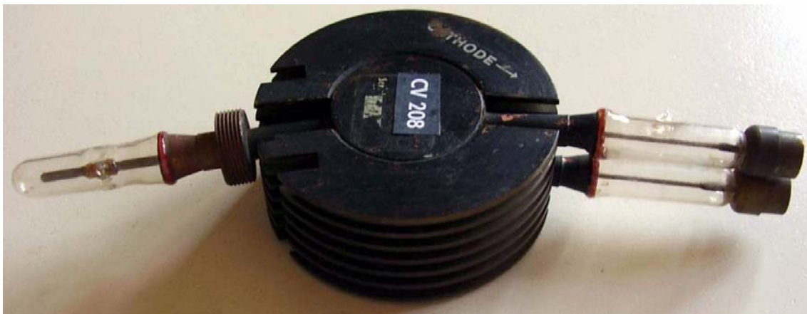
- The collection also include a rare sample of the early production, with separate glass stems for heater and heater / cathode connections.
