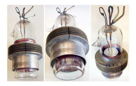
Forced-air cooled UHF pulse transmitting triode. Oxide coated cathode, squirrel-cage grid, external anode with finned heath radiator. This code applies to lower emission NT99, while higher emission units were marked as CV1256.
