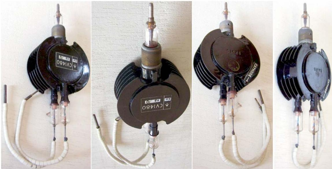
EEV S-band pulse magnetron. Fixed frequency, coaxial output, external magnet.
