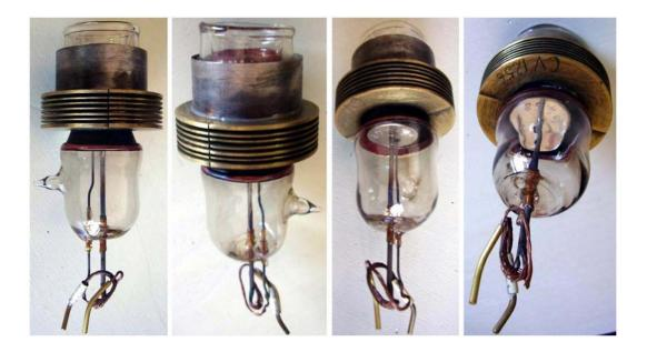
CV1256 was intended for pulsed operation at frequencies up to 600MHz.
