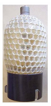
CV125 was a spark gap trigger used in the British radar modulator type 158. Trigatrons, as this family of spark gaps was named, were fired by a trigger electrode through a small hole in the cathode. The textile sock glued over the body was used to prevent glass chips to be scattered all around in case of explosion.
