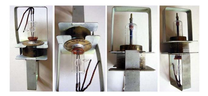
CV1090 is the standardization code for the VT90 early micropup. This sample, still in its shipping frame, was manufactured in Canada by Northern Electric.
