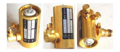
General Electric Microwave Circuit Module, MCM, based upon the GE 14811 planar triode.
