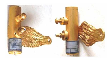
Microwave Circuit Module or MCM by General Electric, based upon the 16841 planar triode.
