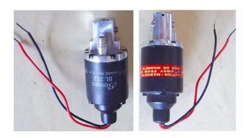
Miniature C-band beacon magnetron. UG-699/U 50 ohms coaxial out connector; heater to flying leads, black lead common to cathode.
