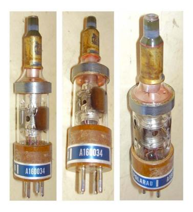
External cavity reflex klystron by Polarad. 6.7 to 11 GHz; 4 pin Peewee base, two contact rings to the external resonating cavity, reflector to the top contact.
