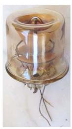
RCA phototube, developed for proximity fuzes. Inverted cone photocathode, ring anode. Two flying leads.
