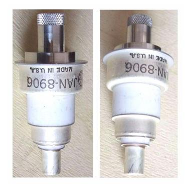
Conduction cooled 8906 and forced-air cooled 8907 are rugged high-reliability UHF power triodes, capable of operation up to 3 GHz. Similar to <u>7815</u> with improved emission, these tubes are intended for pulsed operations in DME transponders or similar airborne equipment. Matrix type cathode for extreme reliability. 8906 is also available as AL selection for airline operations.
