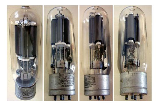
Transmitting triode, graphite anode, 4-pin jumbo base. Used in audio, class A or AB1, amplifier circuits.
