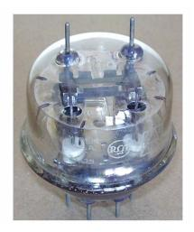
Twin beam power tube capable of operating full-power up to 200MHz and up to 250MHz at reduced power. 15W CGS total tube plate power dissipation. All glass body with septar base.
