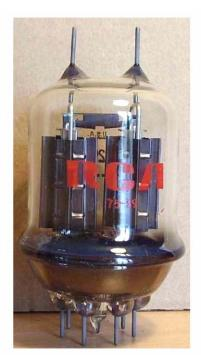
Twin beam power tube capable of operating full-power up to 200MHz and up to 250MHz at reduced power. 30W CGS total tube plate power dissipation; forced-air cooling required. All glass body with septar base.
