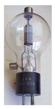
Air-cooled transmitting triode. Thoriated tungsten filament.
