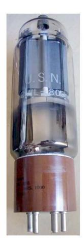
Thoriated tungsten filament requiring 10V at 5A. Giant 5-pin bayonet base. Graphite plate capable of dissipating 125 W, showing a barely perceptible red color.
