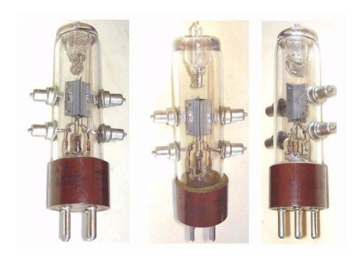
UHF air cooled transmitting triode, capable of operating as oscillator or amplifier. With forced air cooling it can deliver 50W at 400MHz and operate up to 600MHz with reduced power. Four side caps, two for the grid and two more for the anode. The plate shows orange-red color, when tube is operated at full CCS ratings. Based <u>8012</u>.
