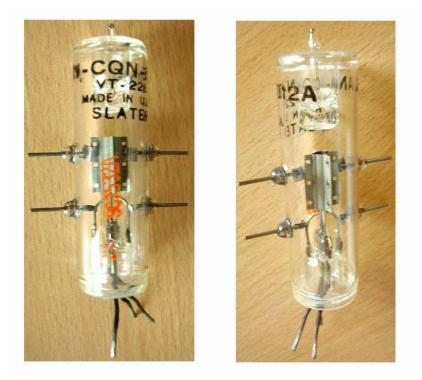
UHF air cooled transmitting triode, capable of operating as oscillator or amplifier. With forced air cooling it can deliver 50W at 400MHz and operate up to 600MHz with reduced power. Four side wires, two for the grid and two more for the anode. Flying wires for heater connections. The plate shows orange-red color, when tube is operated at full CCS ratings. 8012A differs from the <u>8012</u> for using tantalum plate, no visible getter inside the glass bulb. RMA record <u>402</u>.
