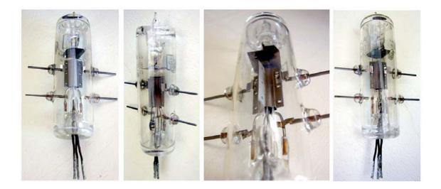
UHF air cooled transmitting triode, capable of operating as oscillator or amplifier. With forced-air cooling it can deliver 50 W at 400 MHz and operate up to 600 MHz at reduced power. Efficiency of about 35% can be expected at 600 MHz. Four side pins, two for the grid and two more for the anode. The plate shows orange-red color, when tube is operated at full CCS ratings. The tube is also known as VT-228.
