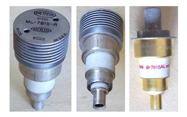
UHF planar power triode, ruggedized variants of 2C39 with ceramic-metal body. Intended for pulse operations in airborne DME or TACAN transponders. Extended grid-to-anode ceramic spacer for improved insulation at high altitudes. Matrix nickel cathode oxide-impregnated for enhanced emission.
