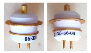
Ceramic-metal planar high-mu triode intended for use as broadband RF amplifier.
