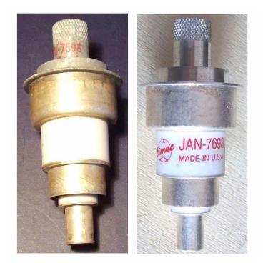
UHF planar power triode, ceramic-metal body derived from the <u>2C39</u> without the heath radiator. Extended grid to anode ceramic spacer for improved insulation at high altitudes. Nickel matrix oxide-impregnated cathode with increased current emission. Intended for pulse applications, such as DME or TACAN transponders. 2.5 kw output pulses at 3 GHz, conduction cooled through fingers all around the anode ring.
