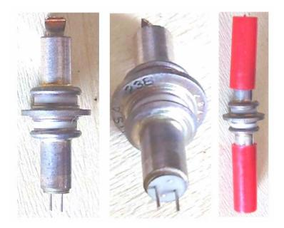
'Pencil' style small-power triode intended for use in airborne transmitting equipment as oscillator, amplifier or frequency multiplier. Planar cermet structure capable of delivering 2.5 W at frequencies up to 5 GHz and higher. 100.000 ft operating altitude.
