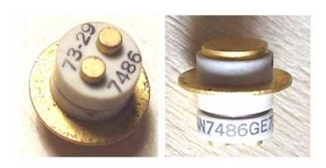
Tiny planar metal-ceramic triode intended for use as oscillator or as RF small-power amplifier in the UHF range.
