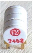
Low-noise triode amplifier. Cermet planar construction, similar to 7077 but with lug terminals for printed circuit mounting.
